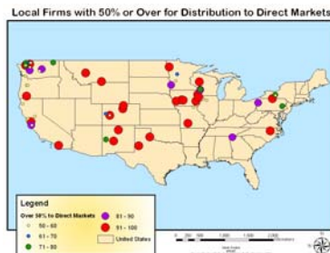
Figure 2- Using colors that do not blend well in combination with graduated symbols makes it hard to discern the point location and attributes. Compare to figure 1.
